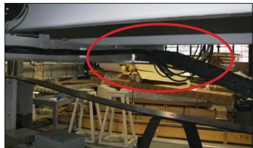
**STEP 4:** Connect the x-axis cables and ground wire to the servomotor above the tool holder angle bracket, secure with wire ties. Reconnect the small cable carrier to the top of the x-axis slide using the screws provided.
